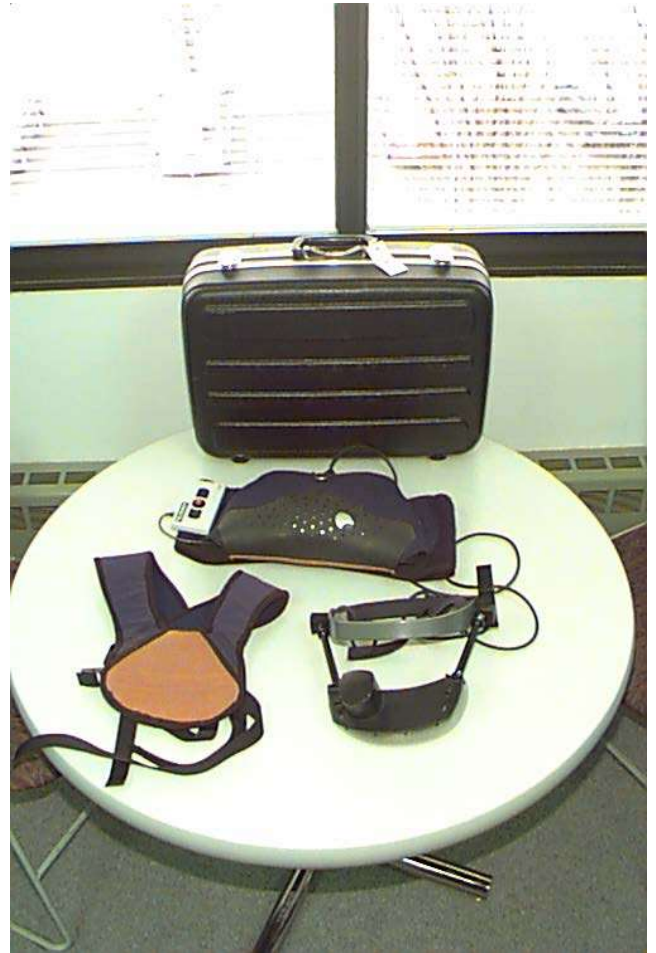
Figure 4.1.8 Wearable Computer with Case
